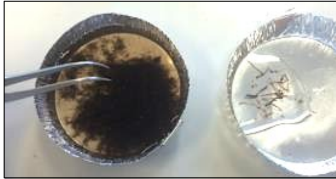
Figure 15. Example of sorting fine root fragments from a dilution subsample ( left ) into a clean ‘root’ tin ( right ). The amount of material in the left tin is a good target when creating dilution subsamples.
