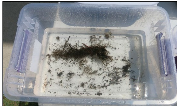
Figure 10. Example of a plastic bin sorting container with a small amount of water to aid root separation.
