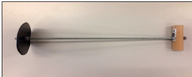
Figure 7. Assembled plunger used to randomize root fragment samples < 1 cm length as part of dilution sampling.
