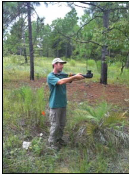
Figure 5. Image of a field researcher acquiring an upward-facing hemispherical photo with the monopod/camera ensemble held at breast height.
