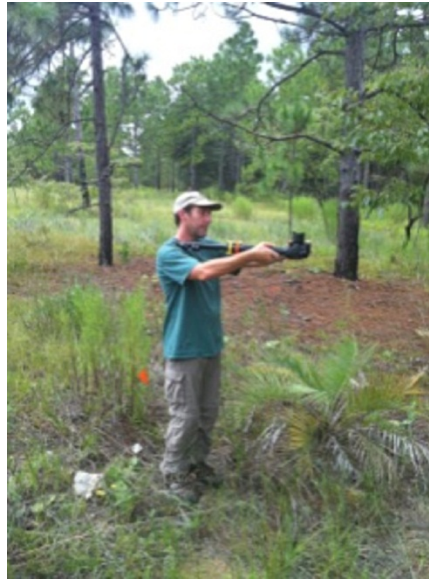
Figure 5. Image of a field researcher acquiring an upward-facing DHP with the monopod/camera ensemble held at shoulder height at the NEON D03 Ordway-Swisher site.
