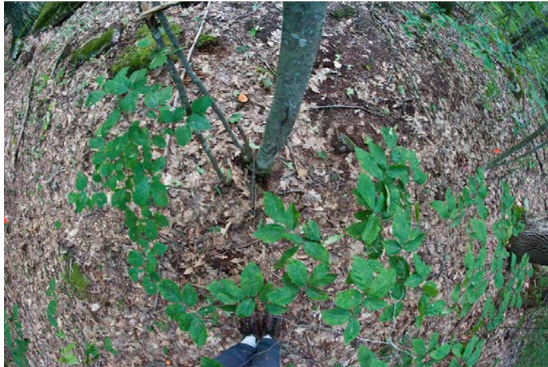
Figure 2. Example of a properly exposed downward-facing DHP at the D01 Harvard Forest site ( photo by B. Chemel ). It is normal for a technician’s feet and a portion of the legs to be included in the photo. These will be masked out during image analysis.
