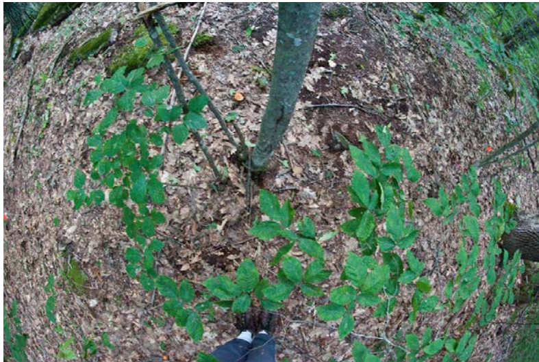
Figure 2. Example of a properly exposed downward-facing DHP at the D01 Harvard Forest site (photo by B. Chemel). Note that green leaves are clearly distinguishable from soil and litter. It is normal for a technician's feet and a portion of the legs to be included in the photo. These will be masked out during image analysis.
