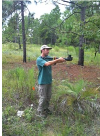
Figure 6. A field researcher acquiring an upward-facing DHP with the monopod/camera ensemble held at shoulder height
