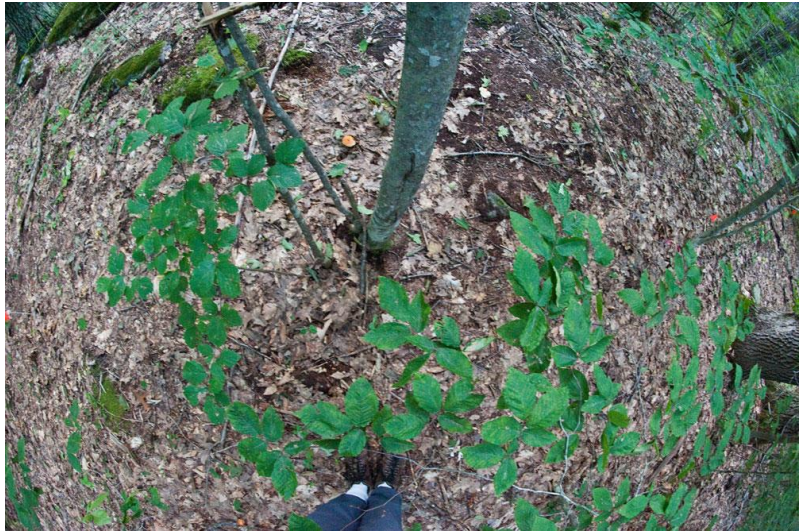
Figure 2. Example of a properly exposed downward-facing DHP at the D01 Harvard Forest site (photo by B. Chemel). Note that green leaves are clearly distinguishable from soil and litter. It is normal for a technician's feet and a portion of the legs to be included in the photo. These will be masked out by the end-user during image analysis.
