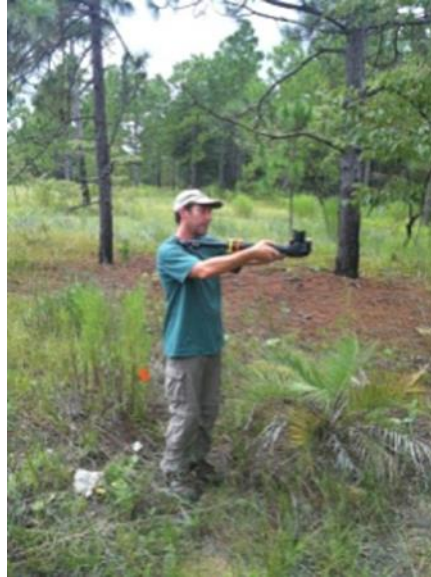
Figure 7. A field researcher acquiring an upward-facing DHP with the monopod/camera ensemble held at shoulder height
