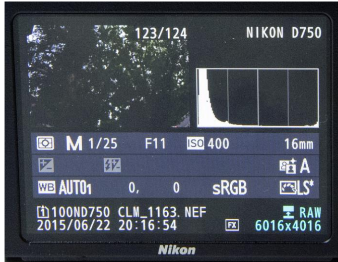
Figure 5. An example of a properly exposed upward-facing DHP, and its associated histogram. Note that the brightest pixels reach the right edge of the histogram, but there is no significant peak at the right.
