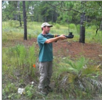
Figure 7. A field researcher acquiring an upward-facing DHP with the monopod/camera held at shoulder height.
