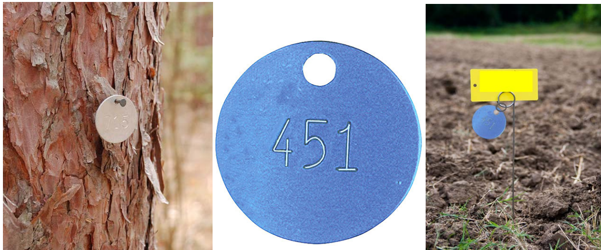
Figure 9. Examples of recommended phenology markers. Photo credit: National phenology network (left), Ben Meadows (center), Forestry Suppliers (right)
