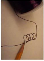
**Figure 5.** Bailing wire coiled around a pencil
