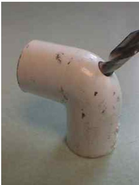
Drill a hole in the back of each 90 degree elbow, as shown.
