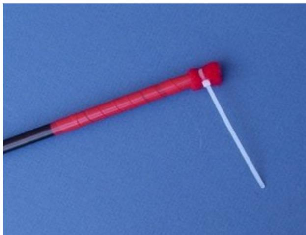
The adhesive back of the Velcro makes it easy to apply. However in the field it will tend to come loose with dirt and moisture. So use a cable tie to hold it on securely.
