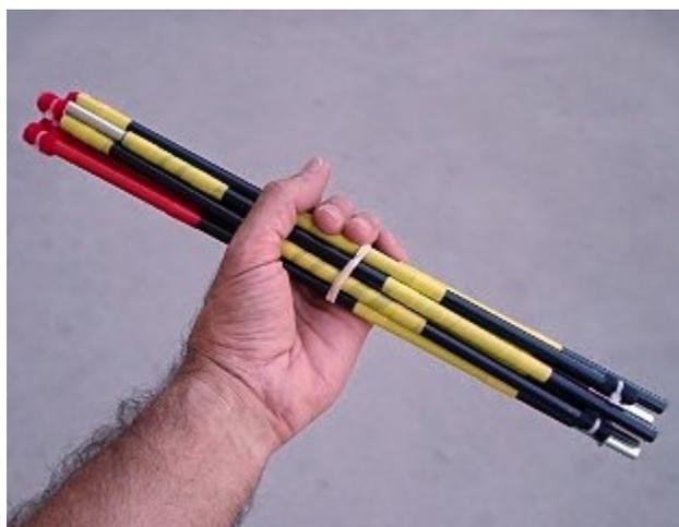
Folded up, the frame makes a small bundle weighing only 300g (aluminum poles) or 240g (fiberglass poles).
