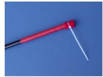
The adhesive back of the Velcro makes it easy to apply. However in the field it will tend to come loose with dirt and moisture. So use a cable tie to hold it on securely.
