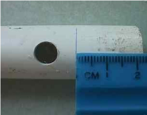
Drill the hole about 33 mm (1-1/4 inch) from one end. This distance is not critical. It must be at least as far as the length that will slip into an elbow, 22 mm (7/8 inch), but it can be as much as 5 - 8 cm (2 - 3 inches).
