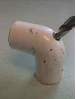
Drill a hole in the back of each 90 degree elbow, as shown.
