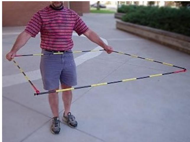
Folded up, the frame makes a small bundle weighing only 300g (aluminum poles) or 240g (fiberglass poles). You can use a leftover piece of the shock cord to make a band to hold the bundle together. If you buy the poles pre-assembled, a rubber band will serve as well.
