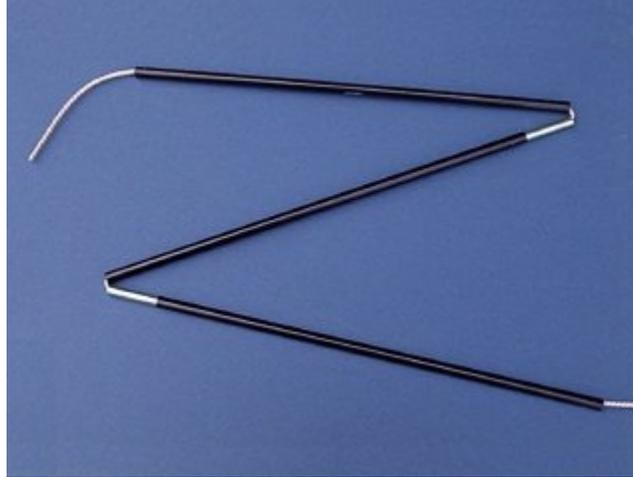
Tie the free end of the cord to a grommet tip. A double half-hitch knot is good. Pull the knot tight to make it as small as possible. It will be a close fit inside the tube. Push the grommet tip down into the tube.
