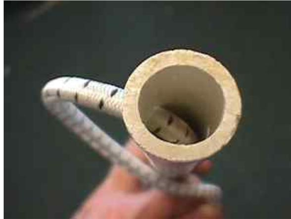
When you have the shockcord through the pipe section and can get enough to work with, thread components together as shown:
