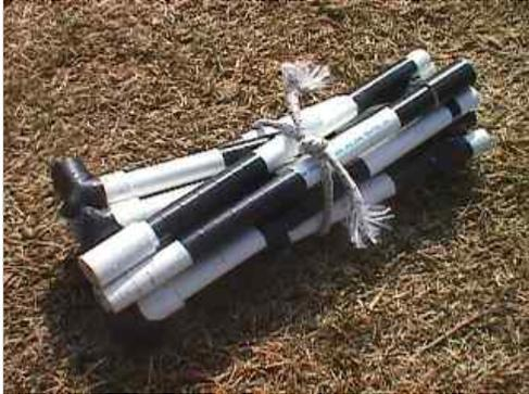
To assemble the frame at a survey site, you push the "empty" end of a bar into the open side of the elbow on another bar. This usually holds together for the minor movements of adjusting the frame position on the ground, but comes apart easily to go around stems and brush.
