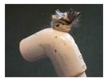
You can test it at this time to see if the tension feels right. You should be able to pull the PVC sections apart easily and fold up the bar. But when straightened out, the shockcord should hold the pieces tight enough together they don't slip apart by accident. There is no need to glue the PVC sections together. When you are satisfied with the tension, you can tighten up the knot and cut the shockcord off to about an inch (few cm).
