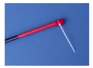
Wrap the rest of the bar in alternating bands of the contrasting color tape. These 10cm bands make it easy to visually estimate percentages within the enclosed one square meter area. Use the brightest colors you can find, to make the frame visually evident in the field and avoid losing it in the brush.
