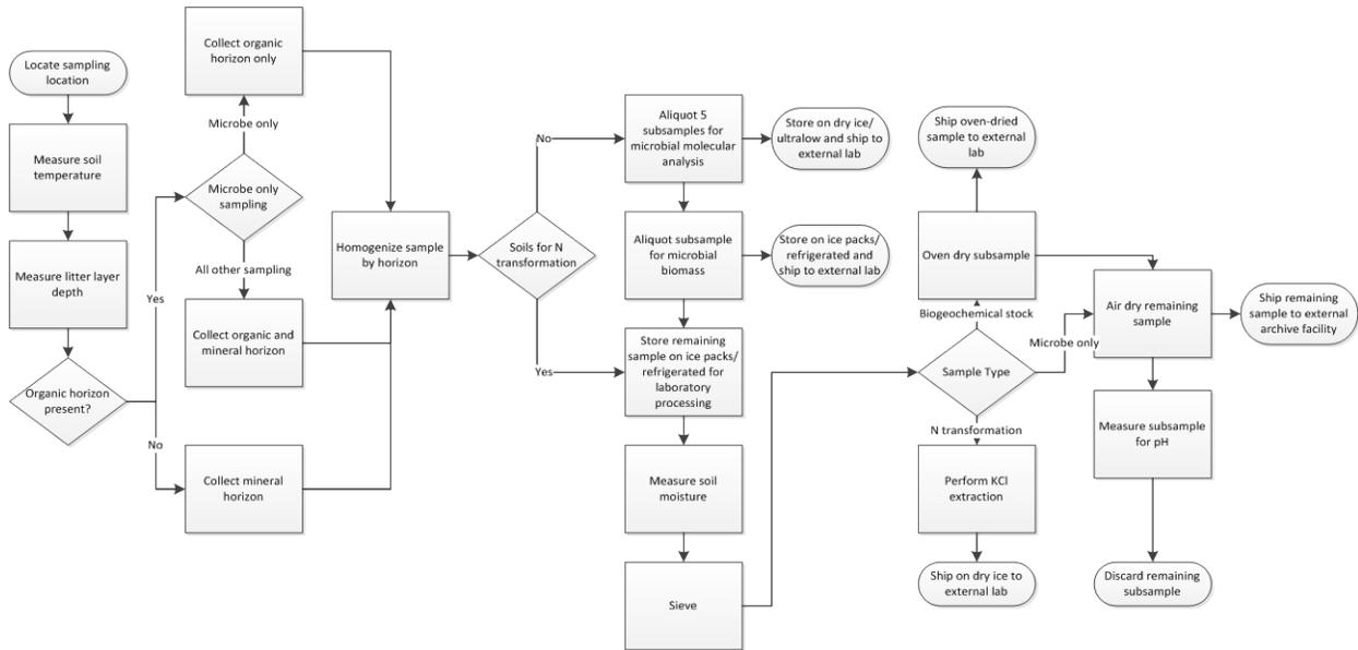
Figure 2 Soil collection, processing and shipping workflow
