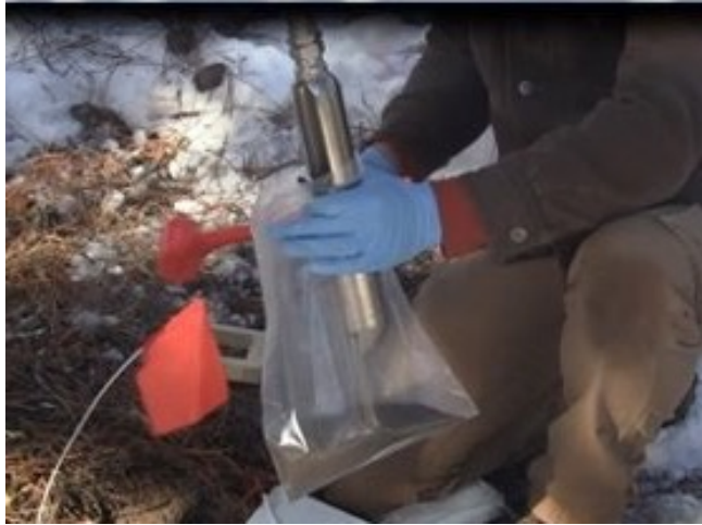
Figure 9. Dispensing soil core into bag for homogenization. Tapping the corer with a rubber mallet can help release soil from the barrel.
