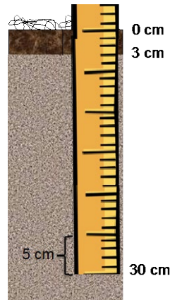
Figure 8 Example soil profile: O horizon sampleTopDepth = 0 cm, sampleBottomDepth = 3 cm; M horizon sampleTopDepth = 3 cm, sampleBottomDepth = 30 cm.
