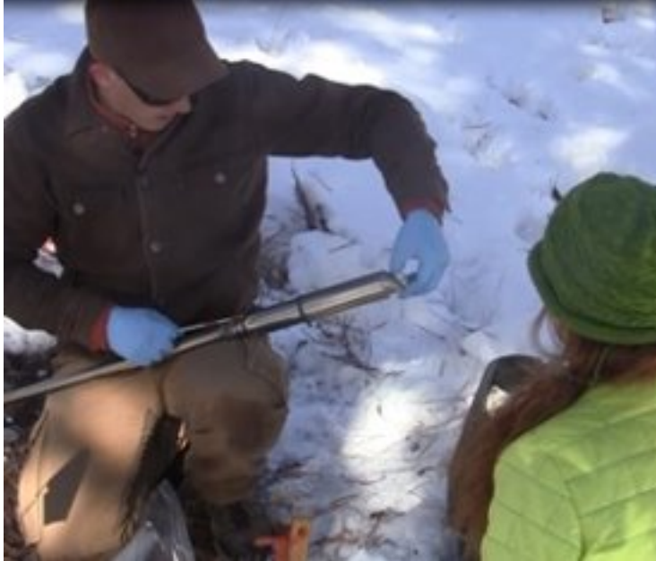
Figure 7. Sterilizing soil auger using chaining pin and 70% ethanol wipe. Gloves should be pre-sterilized.
