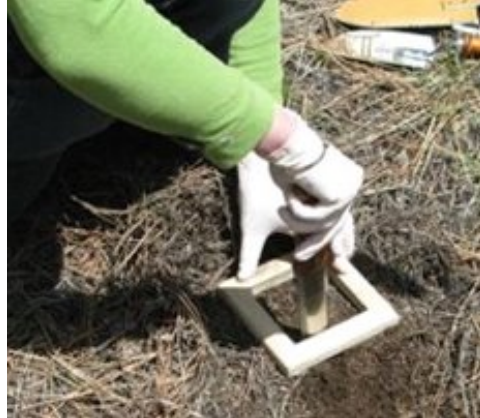
Figure 5. Example use of brownie cutter and hori-hori for O horizon sampling.
