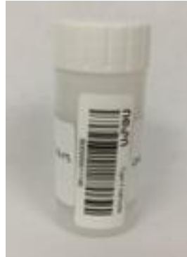
Figure 10. Plastic scintillation vial showing proper orientation of labels. Applies to microbial biomass (-bm), KCl extraction (-kcl), and BGC analysis (-cn) vials.
