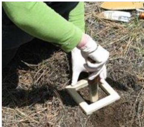
Figure 11. Example use of brownie cutter and hori-hori for O horizon sampling.
