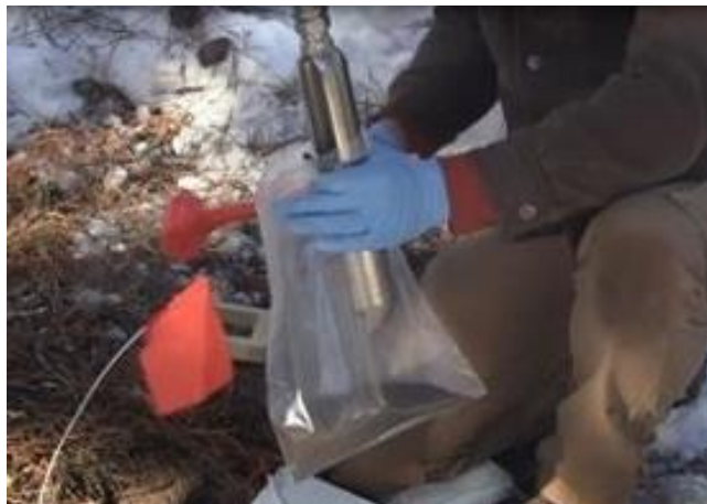
Figure 14. Dispensing soil core into bag for homogenization. Tapping the corer with a rubber mallet can help release soil from the barrel.
