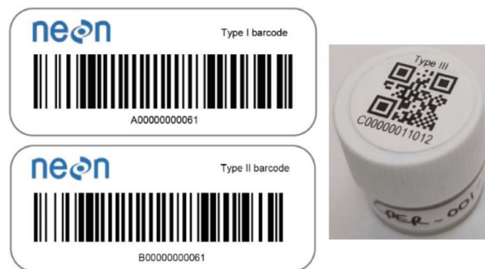
Figure 8. Barcode labels used for the various types of soil samples. Type I barcodes are weatherproof but are not cryo-safe; Type II and III barcodes are cryo-safe and are ideally sized for the sample containers.
