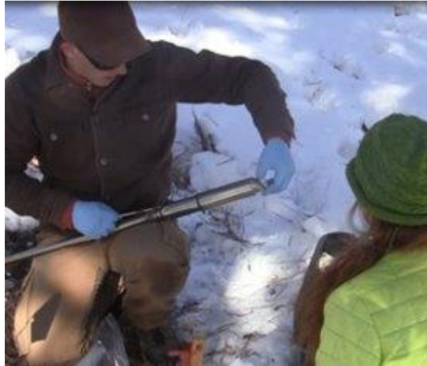
Figure 13. Field staff sterilizing a soil auger using chaining pin and 70% ethanol wipe. Gloves should be pre-sterilized.
