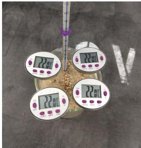
**Figure 7.** Temperature probe calibration setup
