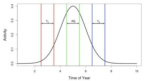
**Figure 2**. Generalized Timing of Soil Sampling. T1 captures the transition from dormancy/low activity to peak activity (PG), while T2 captures the transition from peak activity to dormancy/low activity. The time of year for each sampling period will vary by local geographic and climatic conditions.
