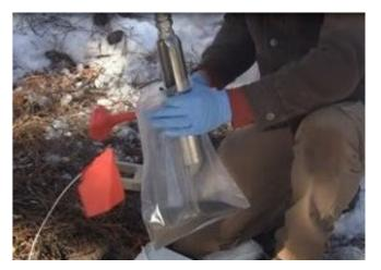
Figure 15. Dispensing soil core into bag for homogenization. Tapping the corer with a rubber mallet can help release soil from the barrel.
