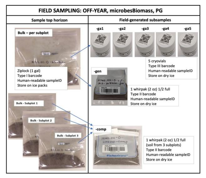
Figure 21. Field-generated samples at Core sites for boutType= microbesBiomass, sampleTiming= peak greenness.
