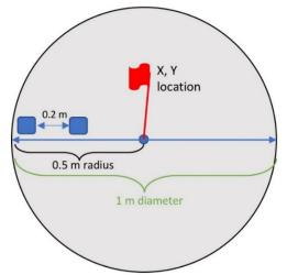
**Figure 16**. Area of acceptable sub-locations for sampling at an X, Y coordinate location. Example cores show ideal distance between initial and final core locations. Locations with rocky soils can use the entire 1 m area, as long as both sub-locations are within 0.5 m of the X, Y location.
