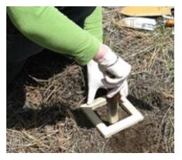
Figure 12. Example use of brownie cutter and hori-hori for O horizon sampling.
