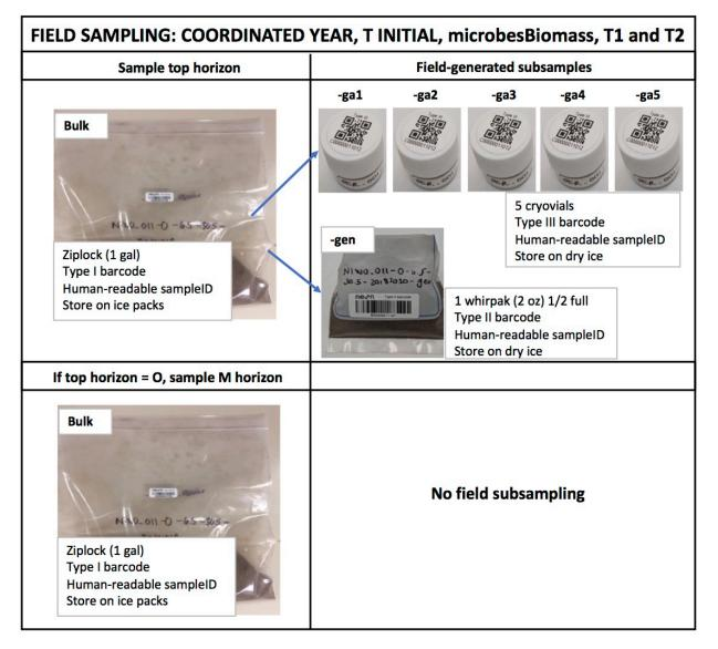
**Figure 23**. Field-generated samples during a Coordinated year for boutType= microbesBiomass, sampleTIming= T1 or T2.
