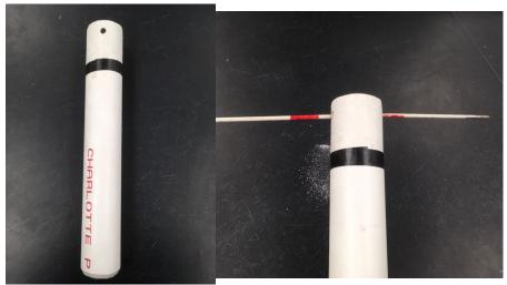
Figure 8. Example coring device used for soil N transformation sampling.
