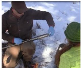
**Figure 14**. Field staff sterilizing a soil auger using chaining pin and 70% ethanol wipe. Gloves should be presterilized.
