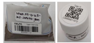
**Figure 13**. Example microbial genetic (-gen, left) and microbial archive (-gaX, right) samples. Microbial metagenomics (-comp) samples will look similar to -gen samples, except for content of the label.
