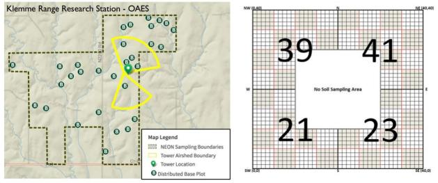
**Figure 1**. *Left*: Example site layout at the OAES field site. Soil sampling occurs at 10 base plots. Four plots are located in the tower airshed and 6 are distributed across the site. *Right*: Gridded plot map for a soil plot. Large numbers centered in each quadrat indicate the subplotID. For each sampling bout, one location is sampled in 3 of the 4 subplots.
