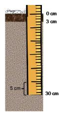
Figure 17. Example soil profile: O horizon sampleTopDepth = 0 cm, sampleBottomDepth = 3 cm; M horizon sampleTopDepth = 3 cm, sampleBottonDepth = 30 cm.
