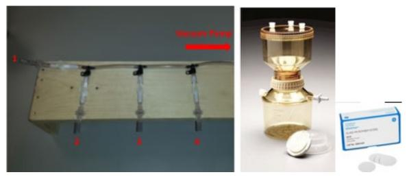
**Figure 18**. Filtration equipment for KCl extractions. Example of a sample manifold set-up (left) and other equipment used for filtration, including filtration unit (extraction funnel + collection cup) and filters (right).
