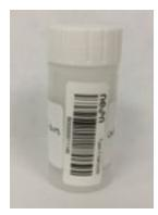
Figure 11. Plastic scintillation vial showing proper orientation of labels. Applies to microbial biomass (-bm), KCl extraction (-kcl), and BGC analysis (-cn) vials.
