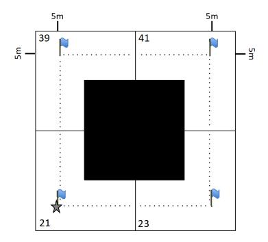
**Figure 19**. Schematic of TOS soil plot demonstrating the general layout of sample locations. Subplot ID's are noted in the left corner of each subplot. Flags denote the corners for the depth transect measuring area, star indicates the location to begin measurement. Dots indicate the general distribution of depth measurements.
