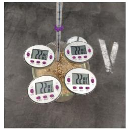
Figure 7. Temperature probe calibration setup
