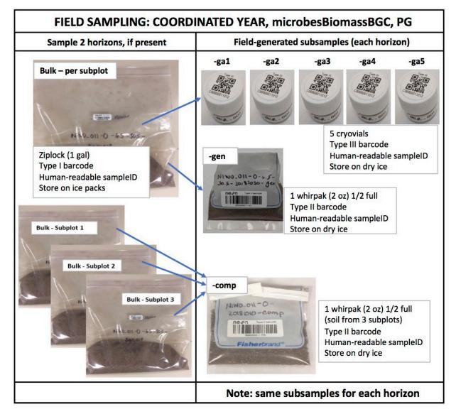
**Figure 24**. Field-generated samples during a Coordinated year for boutType= microbesBiomassBGC, sampleTiming = peak greenness.
