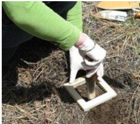
Figure 12. Example use of brownie cutter and hori-hori for O horizon sampling.
