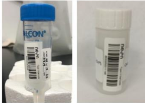
Figure 10. Sample containers illustrating correct orientation of labels. Left: Microbial biomass. Right: KCl extract.
