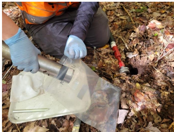
Figure 15. Dispensing soil core into bag for homogenization. For certain soils and sampling devices, tapping the corer with a rubber mallet may be very helpful in releasing soil from the barrel.
