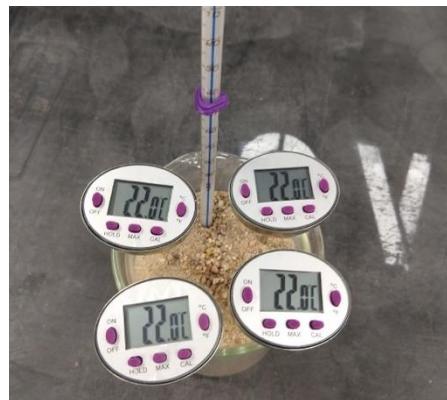
Figure 7. Temperature probe calibration setup.
