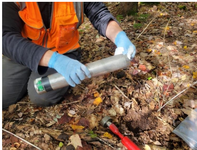
Figure 14. Field staff sterilizing a soil corer using a 70% ethanol wipe. Gloves should be pre-sterilized.
