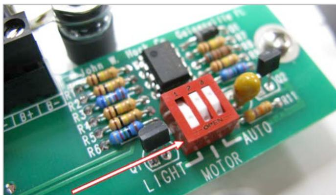
**Figure 5. Picture showing CO2 light trap circuit assembly switches in the closed-open-open position**
