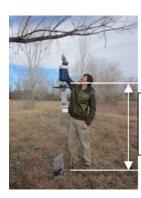
Distance from ground to hole in bottom of cylinder cooler should be 1.5 to 1.8 m
