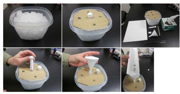
Fig #: example of a chilling station and associated laboratory setup for transferring mosquitoes from catch cups into sample vials.
