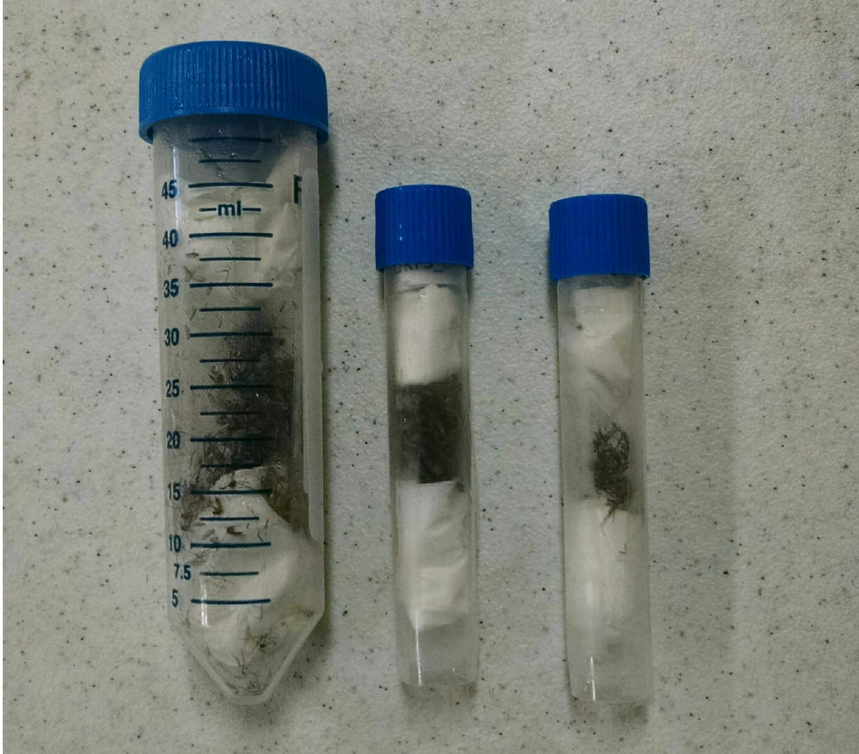
Figure 10 Three mosquito vials. The center vial has an appropriate amount of wadding above and below the sample of mosquitoes. The sample on the left and right have too little material to effectively cushion the sample. Note that the sample ID label is between the upper wadding and the lid of the vial.
