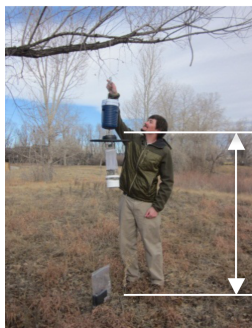
Distance from ground to hole in bottom of cylinder cooler should be 1.5 to 1.8 m
