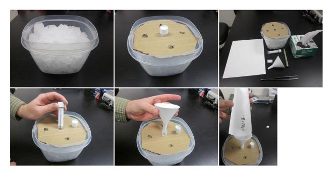
Figure 9 Example of a chilling station and associated laboratory setup for transferring mosquitoes from catch cups into sample vials.
