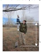
Distance from ground to hole in bottom of cylinder cooler should be 1.5 to 1.8 m
