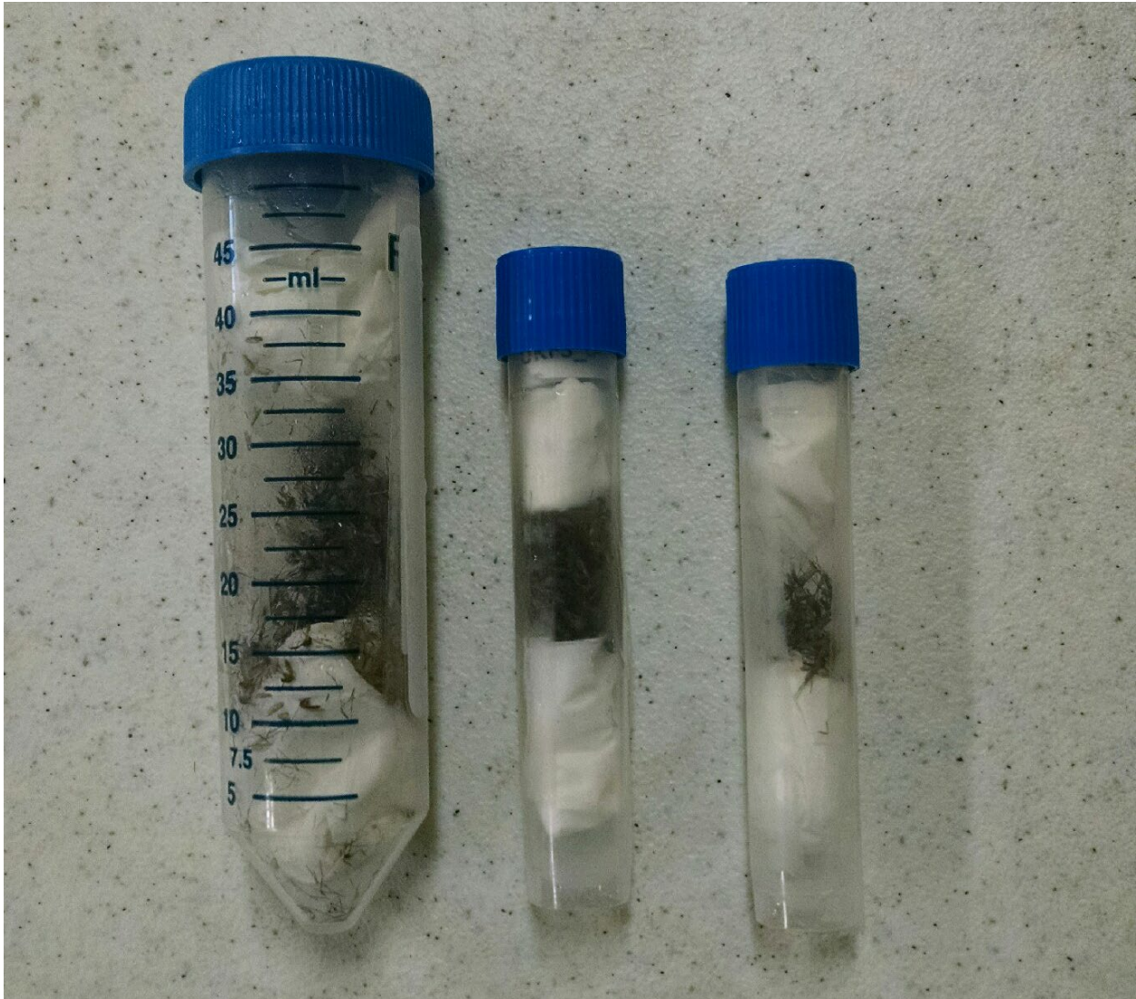
Figure 11 Three mosquito vials. The center vial has an appropriate amount of wadding above and below the sample of mosquitoes. The sample on the left and right have too little material to effectively cushion the sample. Note that the sampleID label must be placed between the upper wadding and the lid of the vial.
