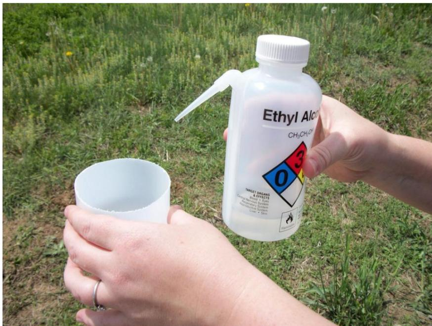
Figure 15. Rinsing sample with 95% ethanol.
