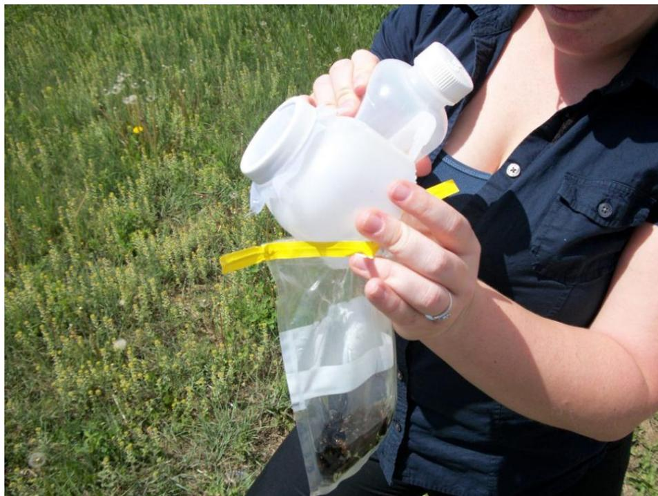
**Figure 17.** Rinsing the sample into the Whirl-Pak and covering sample with 95% ethanol. The mesh is also placed in the bag.
