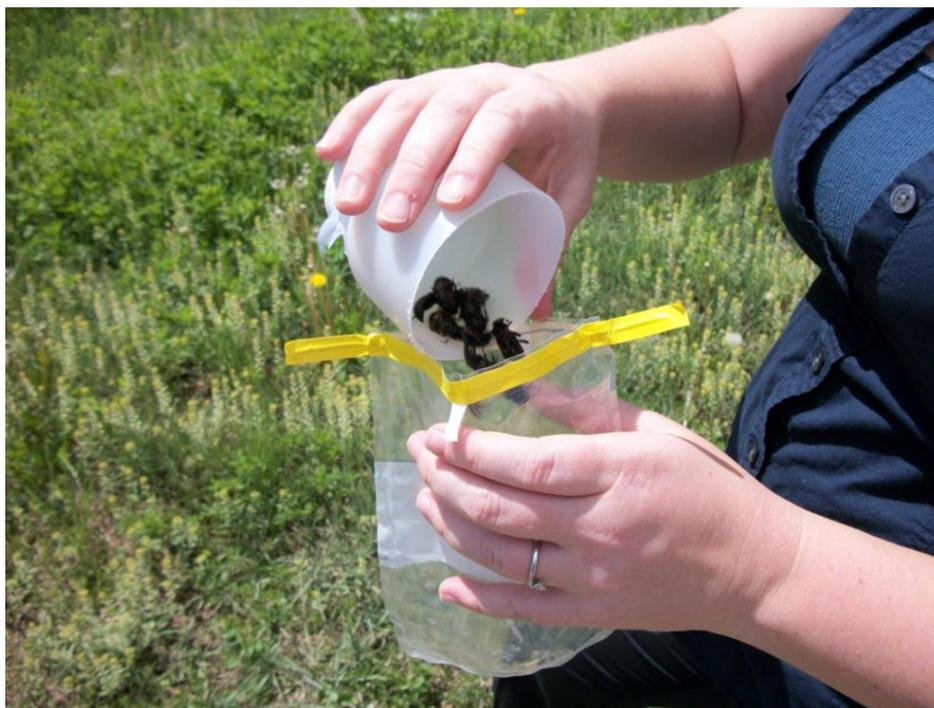
Figure 16. Placing sample in Whirl-Pak bag.
