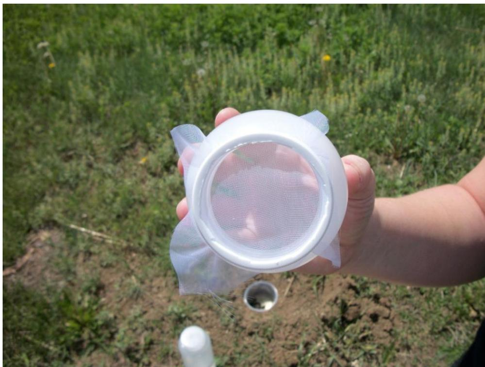
**Figure 9.** A filter installed on a trap bowl.
