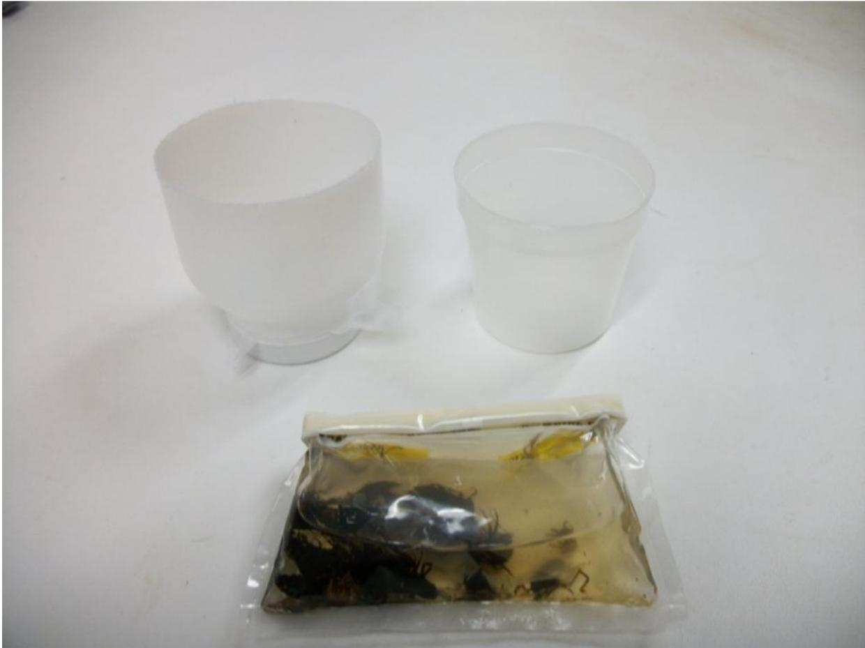
**Figure 21. Preparing for the first ethanol change. Filter cup (sieve) and temporary waste storage container used for sieving sample are shown above the Whirl-Pak.**
