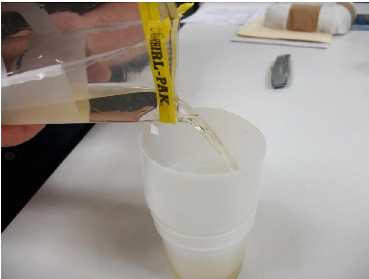
Figure 22. Filtering diluted ethanol off sample into a specimen cup.
