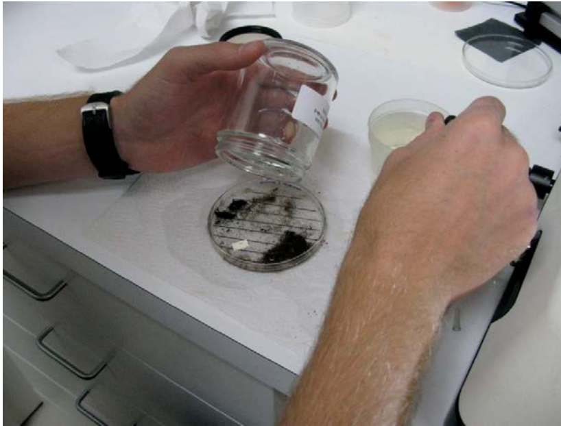
Figure 25. Preparing to sort a sample. Note: technicians will be pouring ethanol and samples from a Whirl-Pak bag and not from a jar.
