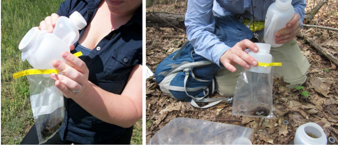
Figure 17. Two alternative ways to rinse the sample into the Whirl-Pak. After rinsing cover the sample with 95% ethanol. The mesh is also placed in the bag.
