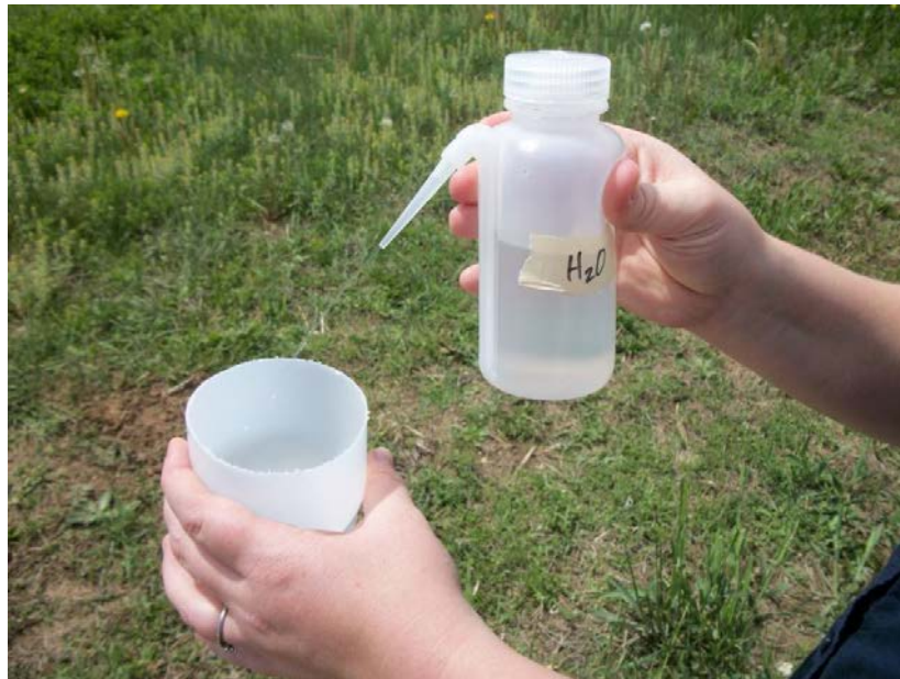
Figure 14. Rinsing sample with water.
