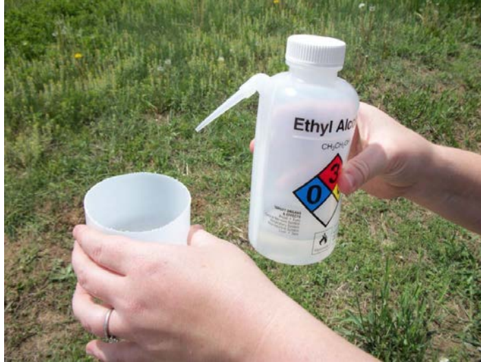
Figure 15. Rinsing sample with 95% ethanol.
