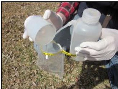
Rinsing filter with ethanol over whirlpak to ensure no organisms are left behind.
