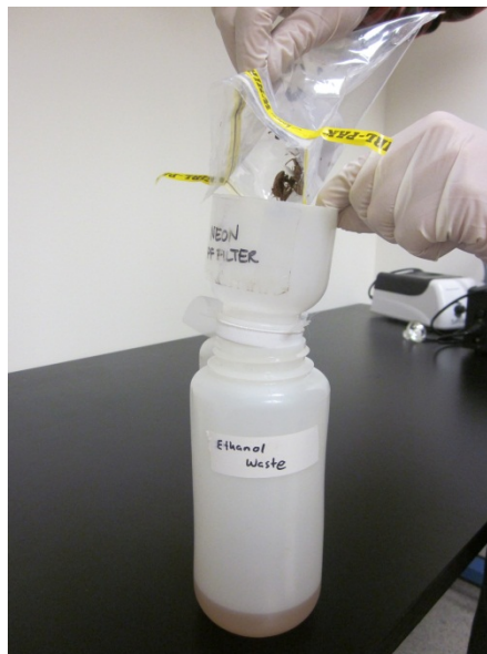
Figure 23. Pouring sample through filter directly into larger waste container.
