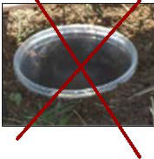
Improperly installed trap. Notice how the lip is above the ground surface.
