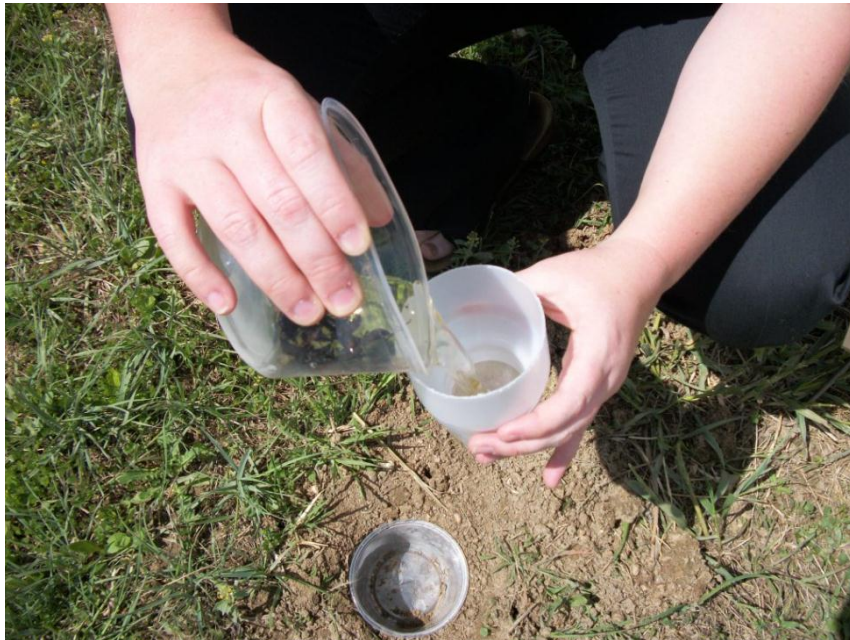
Figure 12. Filtering specimens from trap. The temporary waste container is below the filter (not visible).
