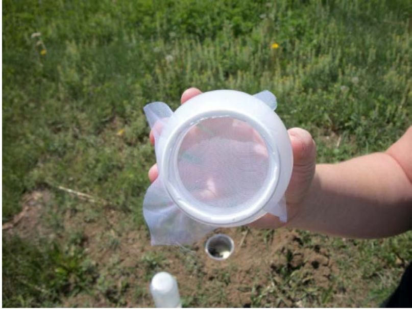
Figure 9. A filter installed on a trap bowl.
