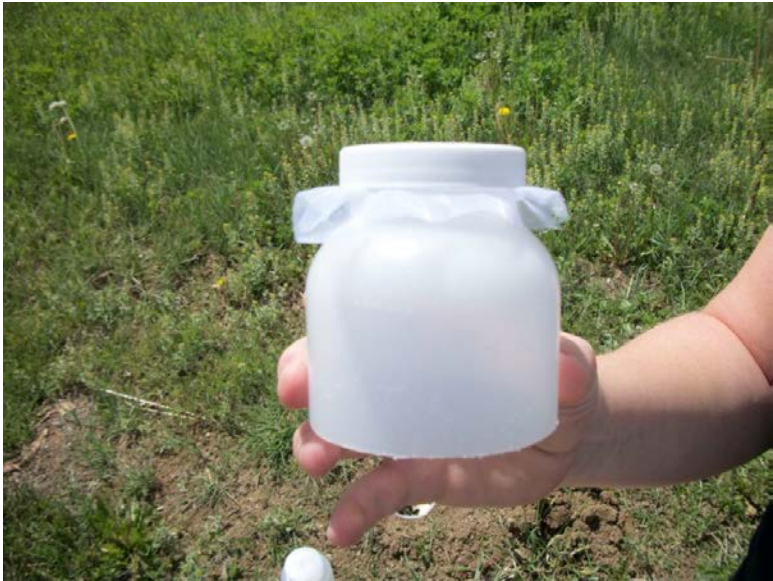
Figure 10. Upside down Nalgene filter ready to use.
