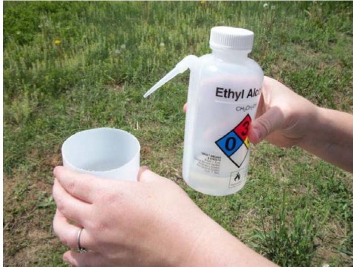
Figure 15. Rinsing sample with 95% ethanol.
