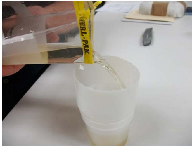
Figure 22. Filtering diluted ethanol off sample into a specimen cup (a temporary waste container).
