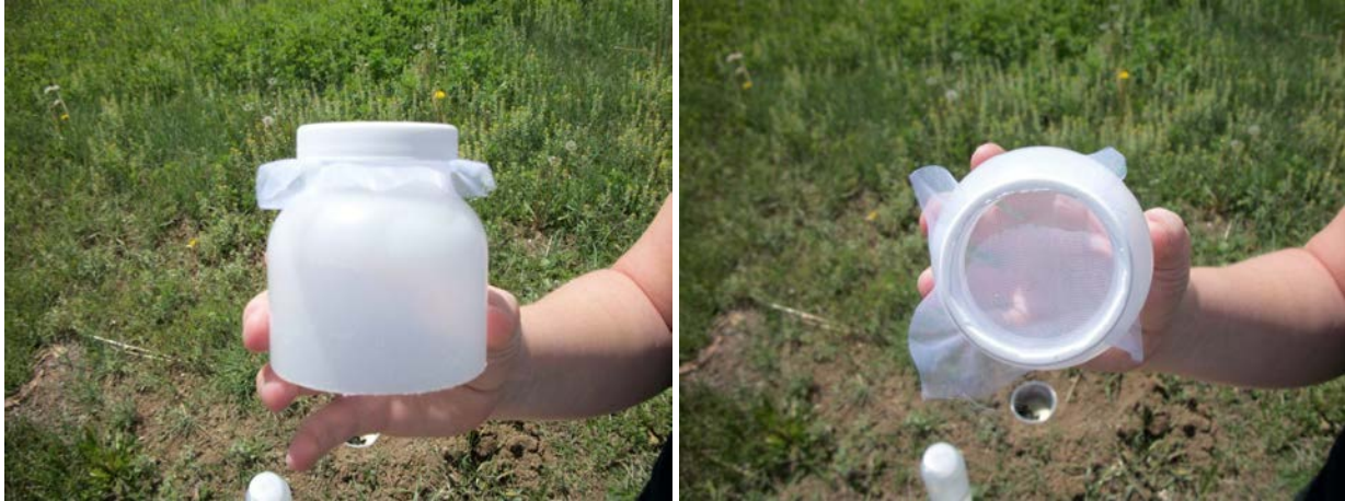
Figure 9. 300 \mu m mesh filter fitted to the top of a Nalgene bottle
