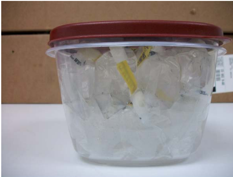
Figure 22. Samples from one sampling bout stored in a sealed container. Label containers using lab tape and permanent markers.
