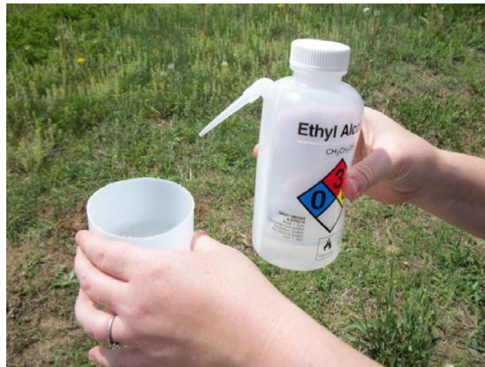
Figure 14. Rinsing sample with 95% ethanol.
