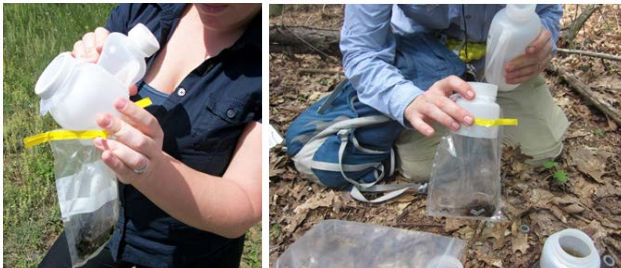
Figure 16. Two alternative ways to rinse the sample into the Whirl-Pak. After rinsing cover the sample with 95% ethanol. The mesh is also placed in the bag.
