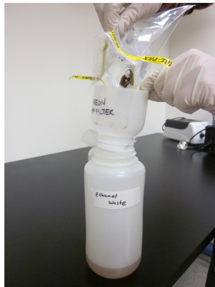
Figure 21. Pouring sample through filter directly into larger waste container.
