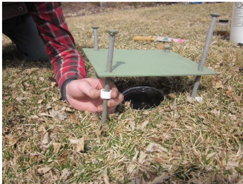
Figure 4. Installing pitfall lid with spacers. Note that the container is flush with the ground.
