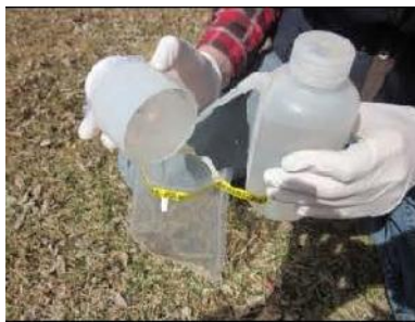
Rinsing filter with ethanol, over Whirl-Pak, to ensure no specimens are left behind
