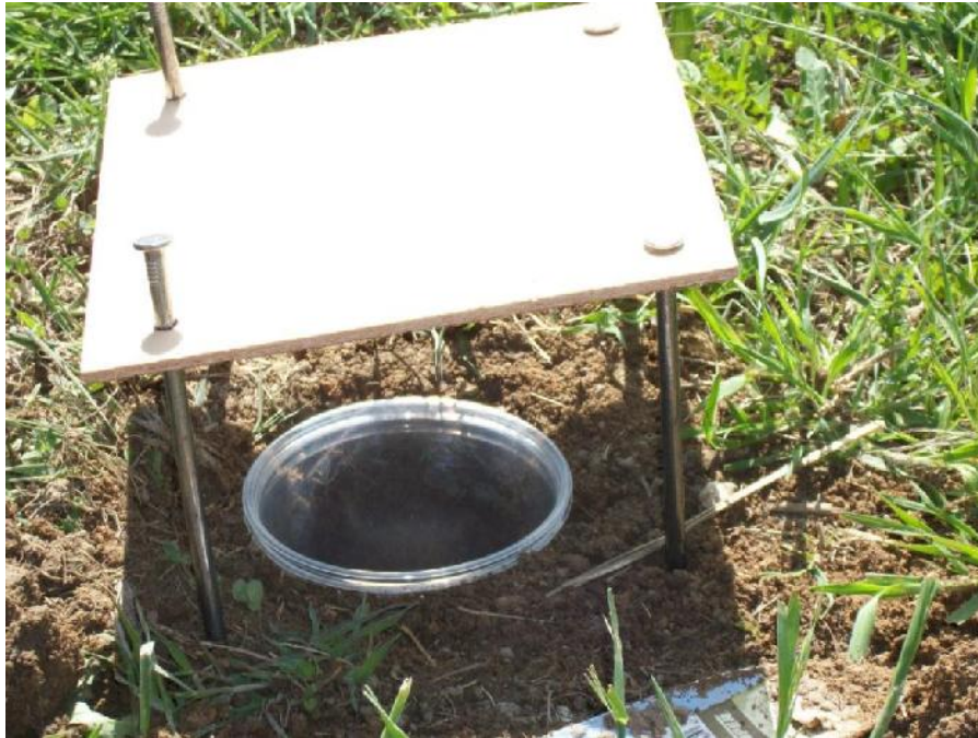
Figure 3. Positioning cover over pitfall trap. Note the pitfall is not sufficiently dug into the ground in this image. The lip should not stick up from the ground.
