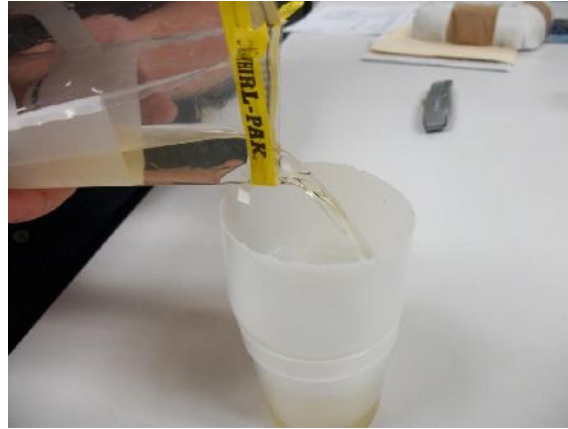
Figure 18. Filtering diluted ethanol off sample into a specimen cup (a temporary waste container).
