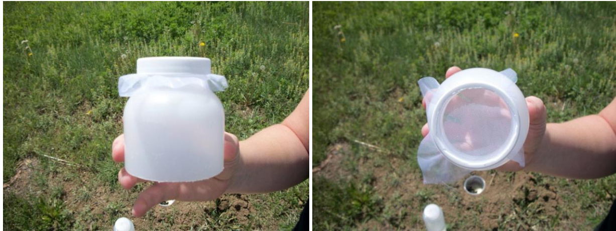
Figure 7. 300 \mu m mesh filter fitted to the top of a Nalgene bottle
