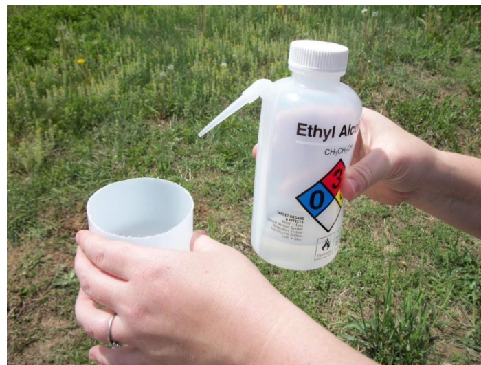
Figure 12. Rinsing sample with 95% ethanol.
