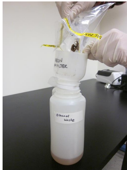
Figure 19. Pouring sample through filter directly into larger waste container.
