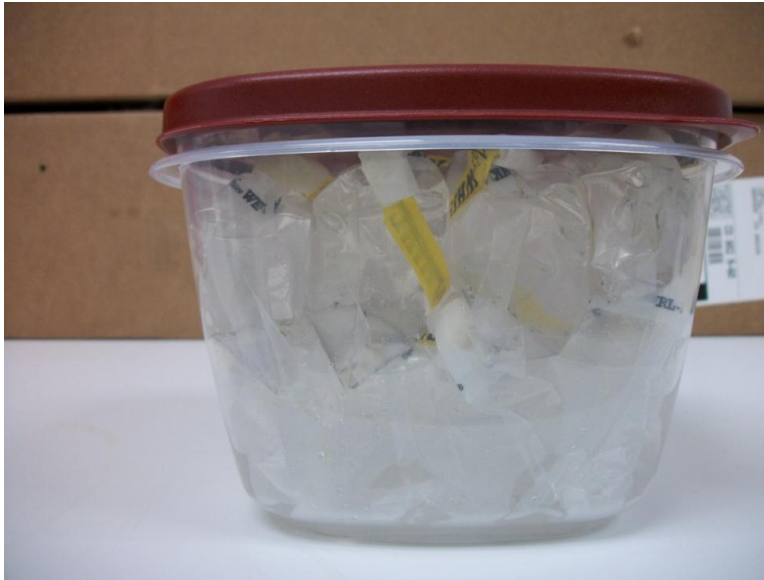
Figure 20. Samples from one sampling bout stored in a sealed container. Label containers using lab tape and permanent markers.
