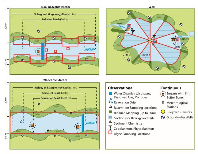
Figure 1: Generic aquatic site layouts for non-wadeable streams/rivers, wadeable streams, and lakes with periphyton, seston, and phytoplankton spatial sampling locations in red.
