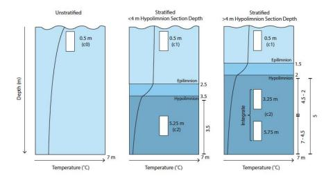
Figure 2: Lake and river sampling depths in non-stratified and stratified water columns.
