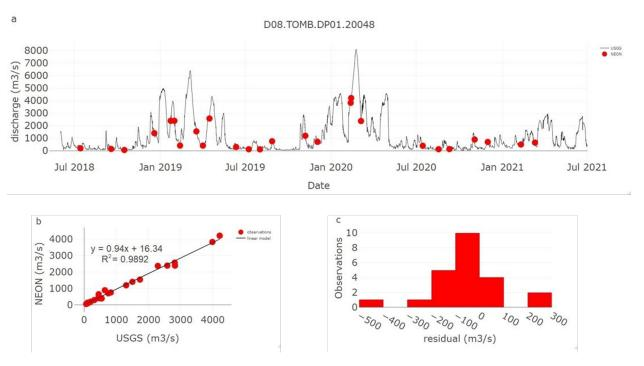
Figure 2: Top panel (a) shows the USGS flow timeseries with red dots for NEON empirical measurements, bottom panel (b) shows a linear regression and equation between USGS data at the time of NEON empirical measurements, and bottom panel (c) shows the distribution of residuals from the regression relationship.
