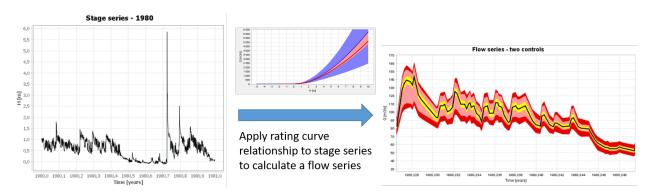
Figure 1: Example stage series and flow series output. Pictures taken from "Stage series" and "Flow series" documentation for BaRatinAGE (Le Coz et al., 2013; Le Coz et al., 2014).
