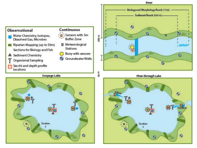
Figure 1: A generic site layout for lakes and rivers with Secchi depth and vertical profile sampling locations (red boxes).
