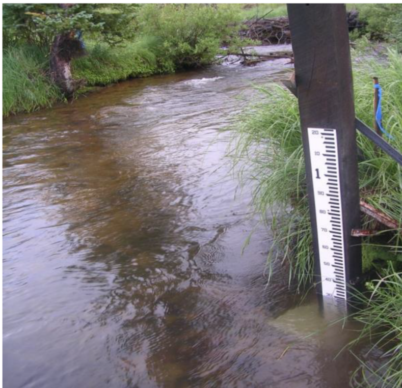
Figure 1: Example of staff gauge installed in a pool
