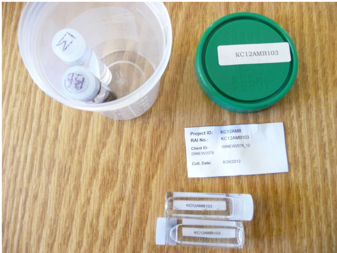
Figure Z. LIMS-generated labels, including RAI number label for specimen cup lid, sample label for inside the specimen cup, and RAI number labels for sample fraction vials.
