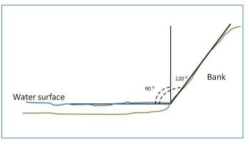
Figure 9. How Bank Angle is Measured
