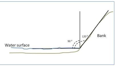
Figure 46 How Bank Angle is Measured
