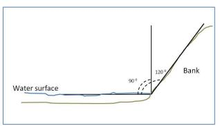
Figure 64 How Bank Angle is Measured
