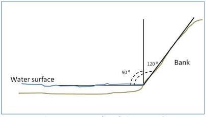
Figure 42. How Bank Angle is Measured
