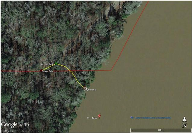
**Figure 36** Map showing the location of power pole, the Aquatic and Auxiliary Portal for D08 Lower Tombigbee River, the clearing required (red box) and the conduit run (yellow).
