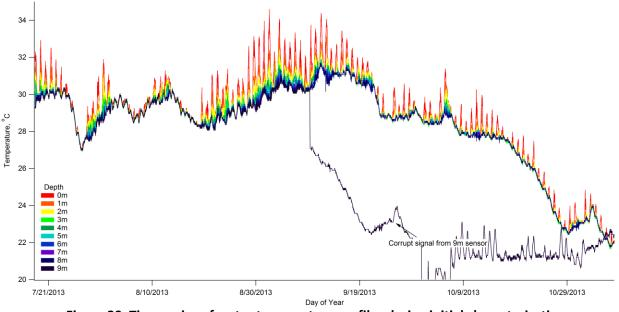
Figure 29. Time series of water temperature profiles during initial characterization.
