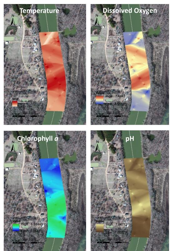
Figure 36. Interpolated surfaces of water quality data from transects performed along the reach.
