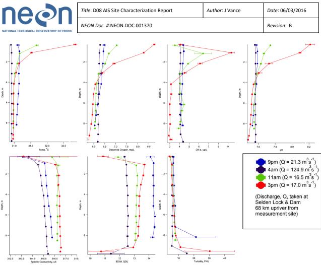
Figure 35. Water quality profiles over a daily cycle taken to investigate the spatiotemporal variability of biogeochemical cycles.
