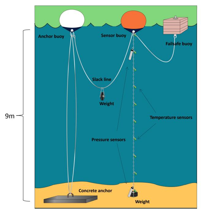
Figure 28. Schematic of moored buoy used to measure temperature profile at Black Warrior River.
