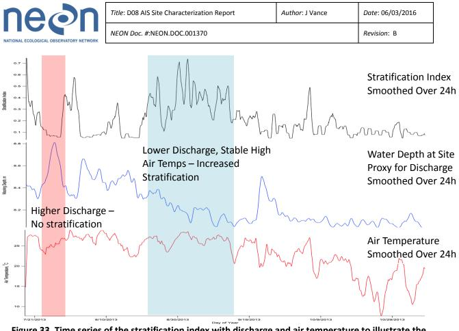
Figure 33. Time series of the stratification index with discharge and air temperature to illustrate the physical drivers of variability.
