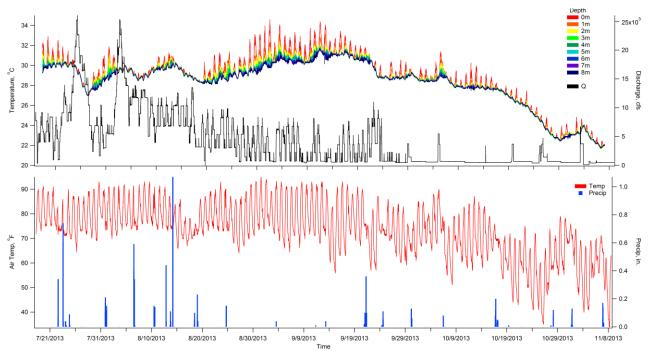
Figure 32.Time series of water temperature profile with discharge (top) and air temperature with precipitation (bottom) during initial characterization.
