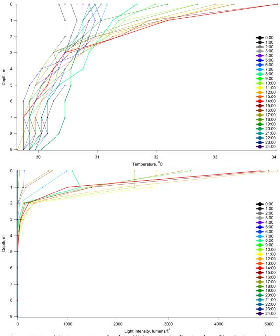
Figure 31. Overlain temperature (top) and light intensity (bottom) profiles during peak stratification.
