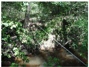
Figure 58 Typically, at least one bank steeply rises ~2 m from the channel to the floodplain. Shown here is the right bank of the Mayfield Creek (STR) S1 location.
