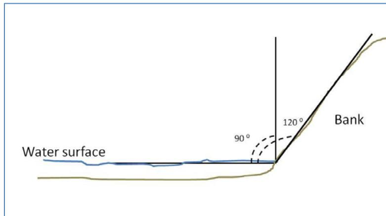
**Figure 25** How Bank Angle is Measured
