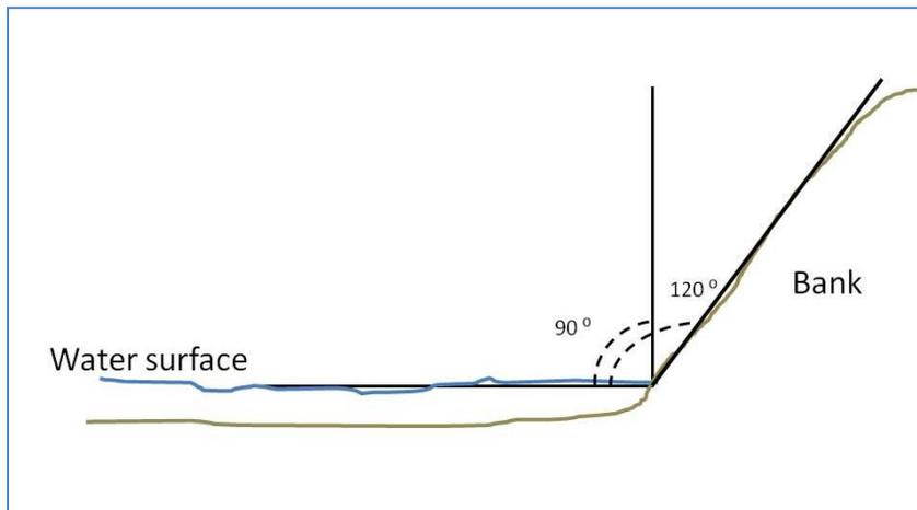
**Figure 36** How Bank Angle is Measured
