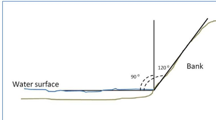
**Figure 8** How Bank Angle is Measured
