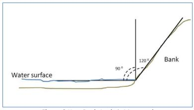
Figure 8 How Bank Angle is Measured
