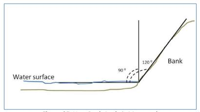
Figure 25 How Bank Angle is Measured
