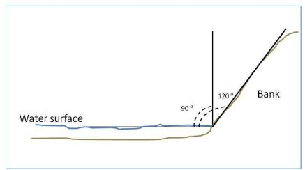
Figure 36 How Bank Angle is Measured
