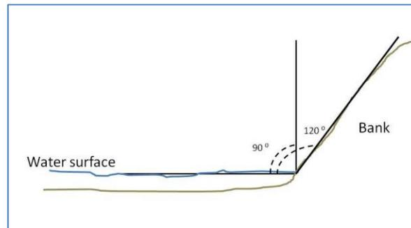
**Figure C7** How Bank Angle is Measured
