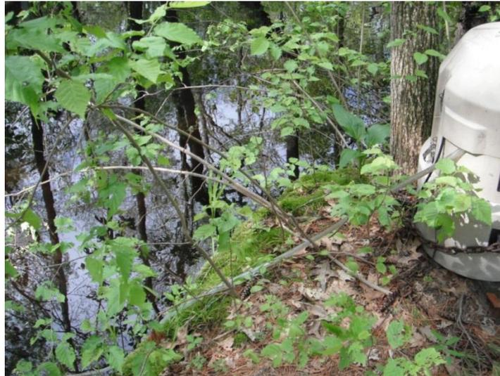
**Figure D10** a) Nutrient autosampler (Wil Wolheim, UNH) on left bank between S1 and S2. B) Nutrient autosampler sampling tube extending into the stream.
