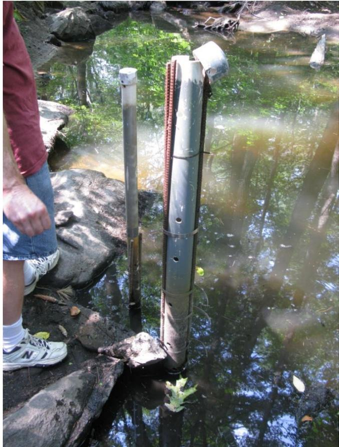
**Figure D9** Stream gage installed by UNH (Wil Wolheim) on the left bank between S1 and S2. Well contains a pressure transducer.
