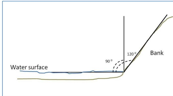
**Figure D7** How Bank Angle is Measured
