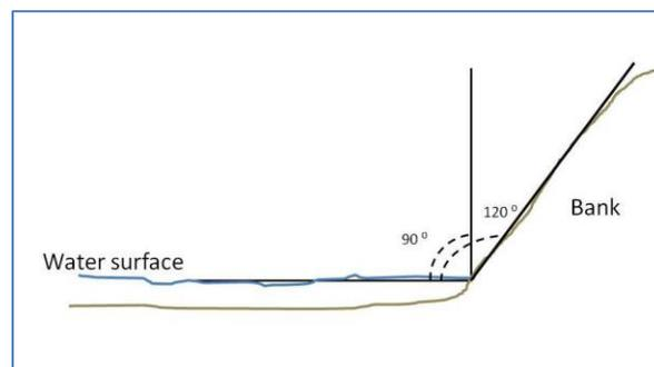
**Figure 7** How Bank Angle is Measured
