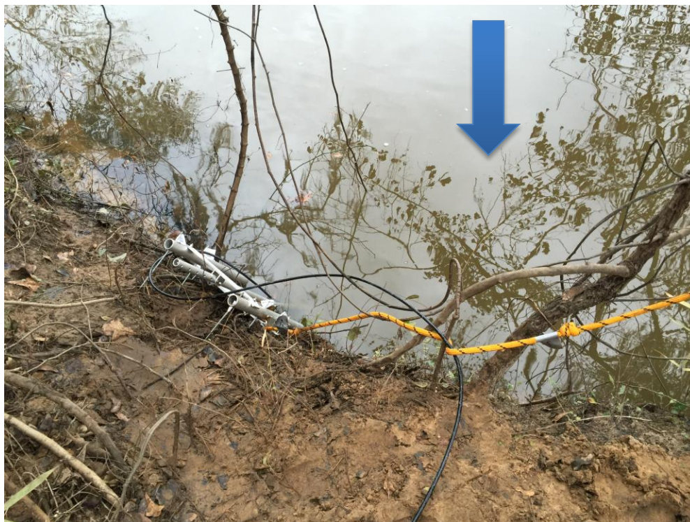
Figure 32 Picture of location of the level gage. (shows temporary infrastructure for deploying ADCP used to measure discharge and velocity fields.)
