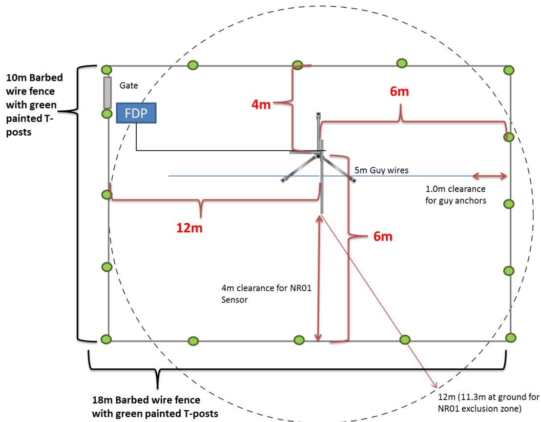
**Figure 20.** Schematic showing the cattle fencing required for met station and associated FDP at Prairie Lake.
