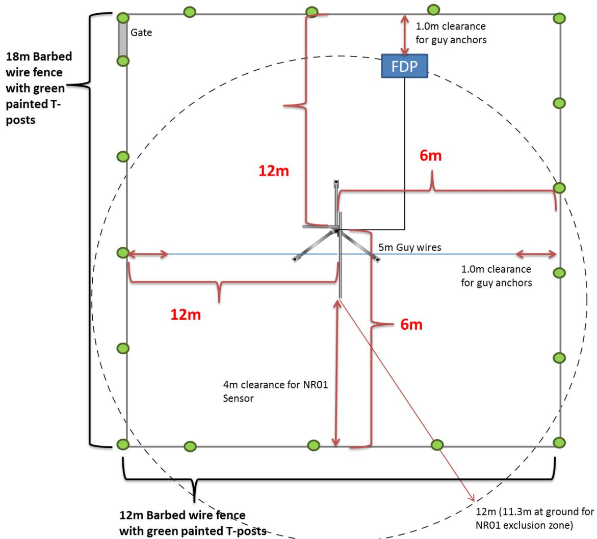
**Figure 5.** Schematic showing the cattle fencing required for met station and associated FDP at Prairie Pothole.
