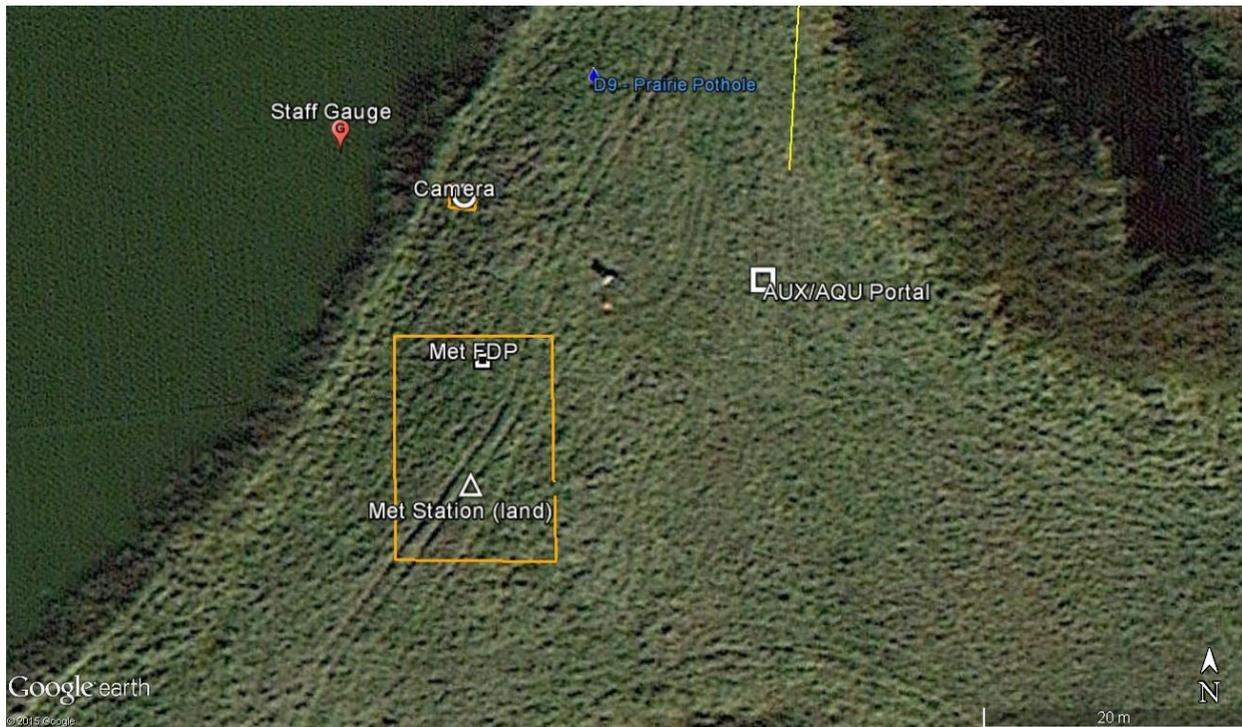
**Figure 4.** Google imgae showing the fencing in yellow required to enclose the both the met station and associated FDP and separately the camera.
