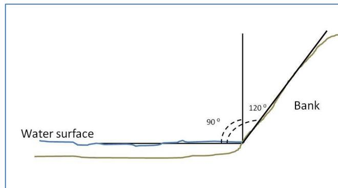
**Figure 9.** How Bank Angle is Measured
