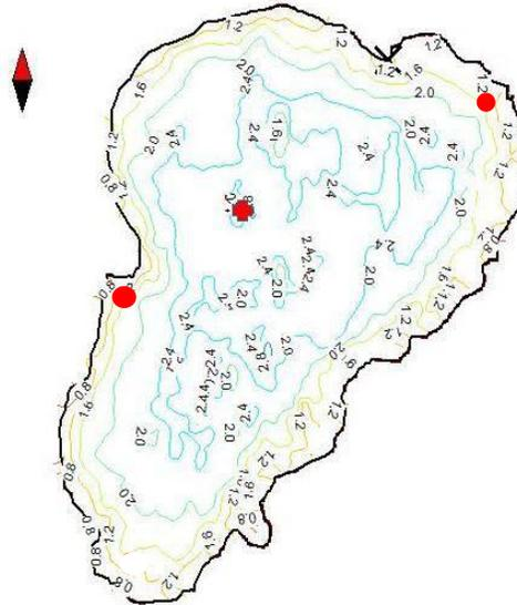
**Figure 3.** Bathymetric map of D09 Prairie Pothole. The red cross denotes the location of S1 and co-located met station. The red circles denote the location of inlet and outlet sensor infrastructure.
