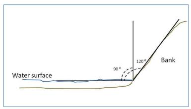
Figure 23. How Bank Angle is Measured
