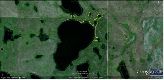
Figure 15. Expected flood zones (yellow line) on the N-NE side of D9 Prairie Pothole. This area should not be used for infrastructure that is sensitive to water or needs to be accessed regularly due to likely flood conditions.
