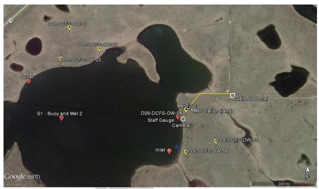
**Figure 17.** Google earth image of D09 Prairie Pothole Denoting Draft Locations of Buoy (S1 and Met 2), the inlet and outlet, land-based met station, staff gauge, camera and field device post (FDP)..
