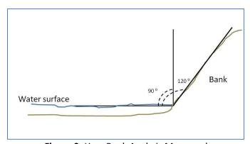
Figure 9. How Bank Angle is Measured
