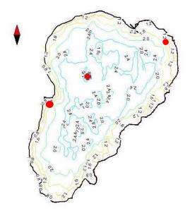
**Figure 3.** Bathymetric map of D09 Prairie Pothole. The red cross denotes the location of S1 and colocated met station. The red circles denote the location of inlet and outlet sensor infrastructure.
