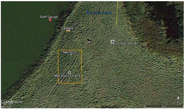
**Figure 4.** Google imgae showing the fencing in yellow required to enclose the both the met station and associated FDP and separately the camera.
