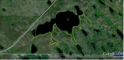
**Figure 26.** Expected flood zones (yellow line) on the S side of D9 Prairie Lake. This area should not be used for infrastructure that is sensitive to water or needs to be accessed regularly due to likely flood conditions.
